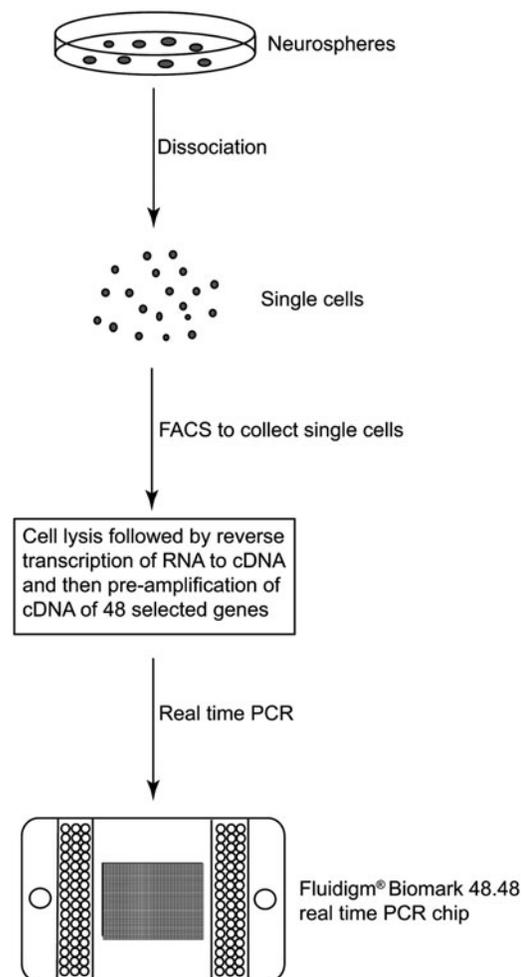
**FIG. 1.** Workflow for single-cell mRNA profiling. Neurospheres are dissociated into single cells and sorted by FACS. Each sorted cell is then lysed before reverse transcription and real-time PCR are performed on the single cells to analyze the expression of 48 selected genes. FACS, fluorescence-activated cell sorting; PCR, polymerase chain reaction.
